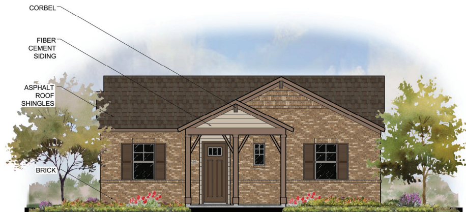
Front Elevation Elevation B 1/4" = 1'-0"
