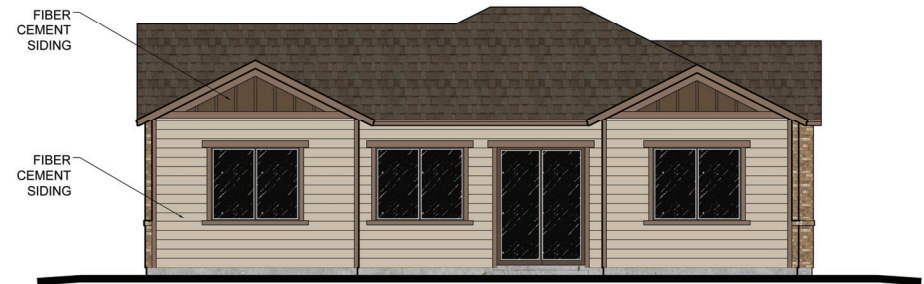
Rear Elevation Elevation B 1/4" = 1'-0"
