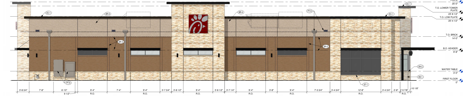
REAR ELEVATION - WEST (PRIMARY FACADE) 3/16" = 1'-0"
