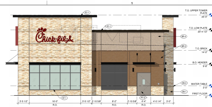
C2 FRONT/SIDE ELEVATION - NORTH (PRIMARY FACADE)
