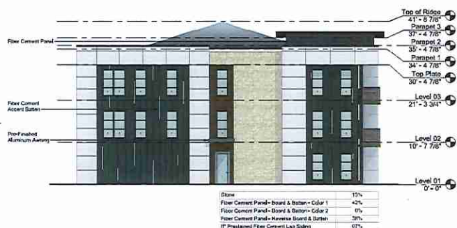
13 Building 3 - North Elevation Scale: 1" = 10'-0"
