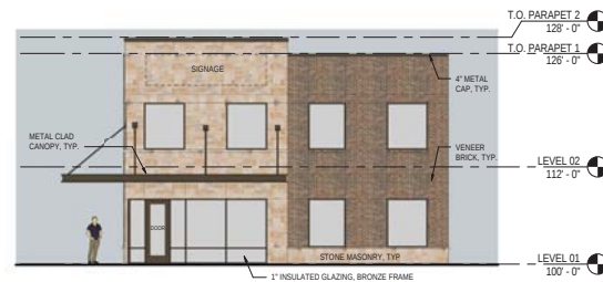
5 EXTERIOR ELEVATION - SOUTH 1/8" = 1'-0"
