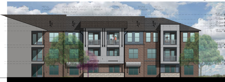
04 EXTERIOR ELEVATION SCALE: 3/32" = 1'-0"
