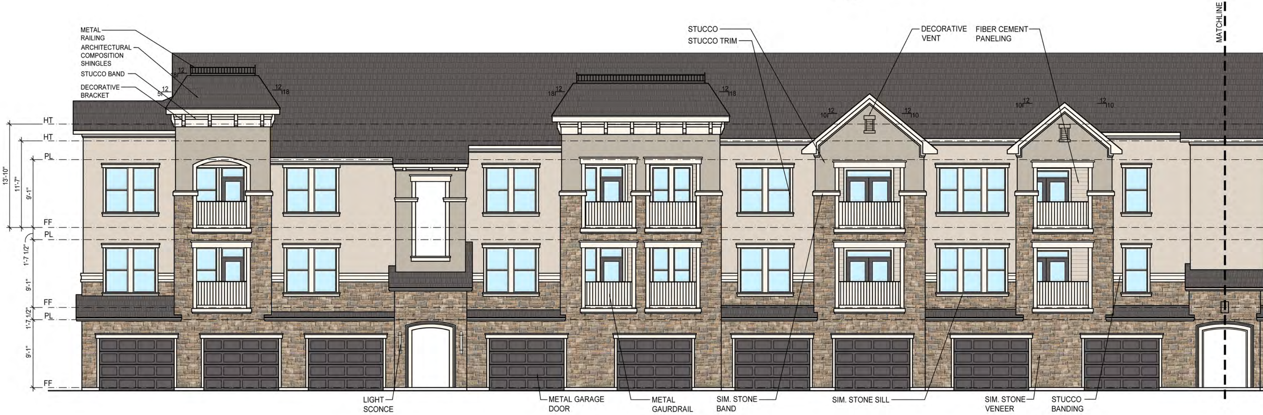
02 BUILDING "G" - FRONT ELEVATION 1/8" = 1'-0"
