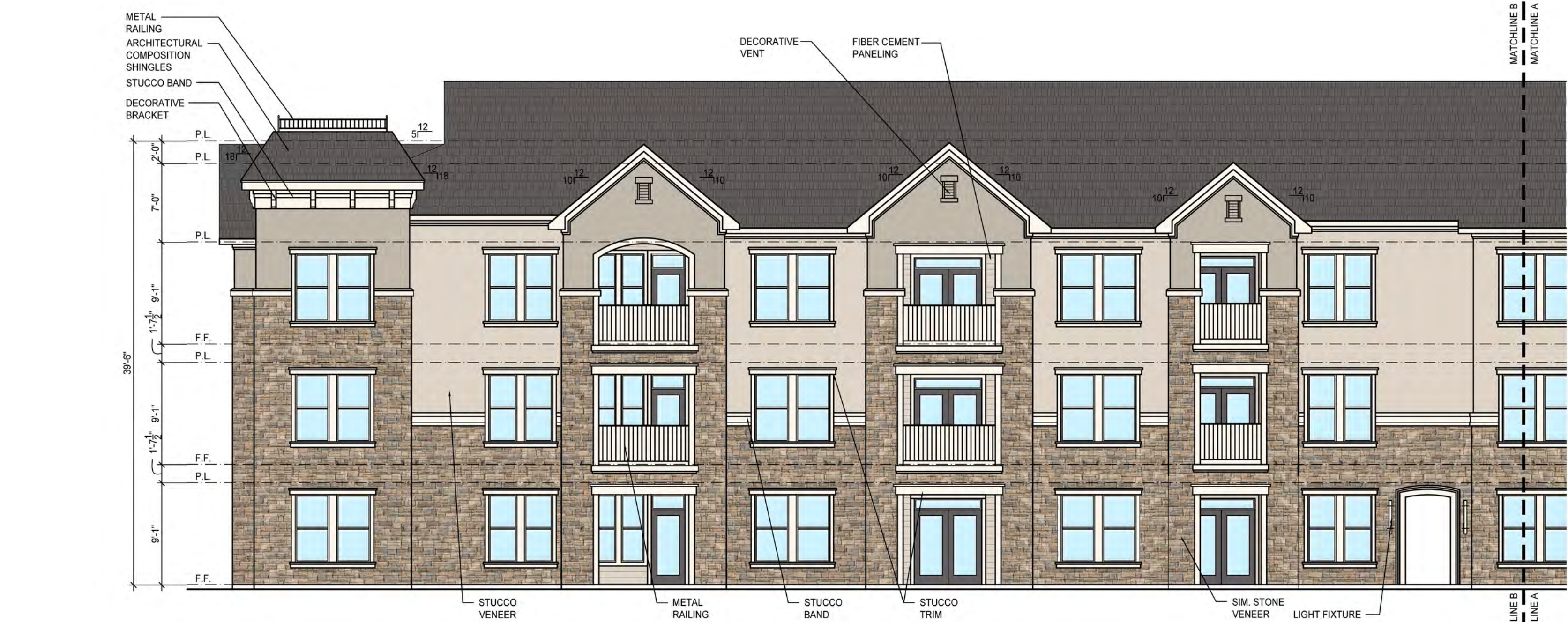
02 BUILDING "C" - REAR ELEVATION 1/8" = 1'-0"
