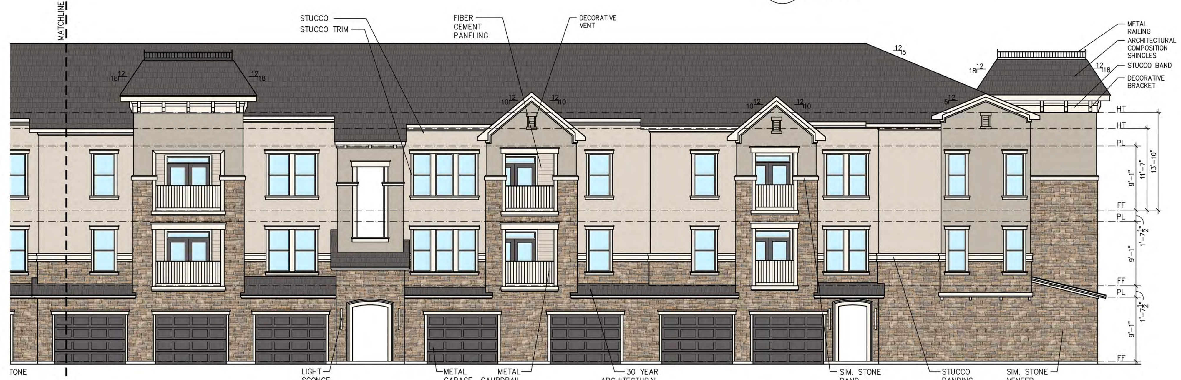
02 BUILDING "F" - FRONT ELEVATION 1/8" = 1'-0"
