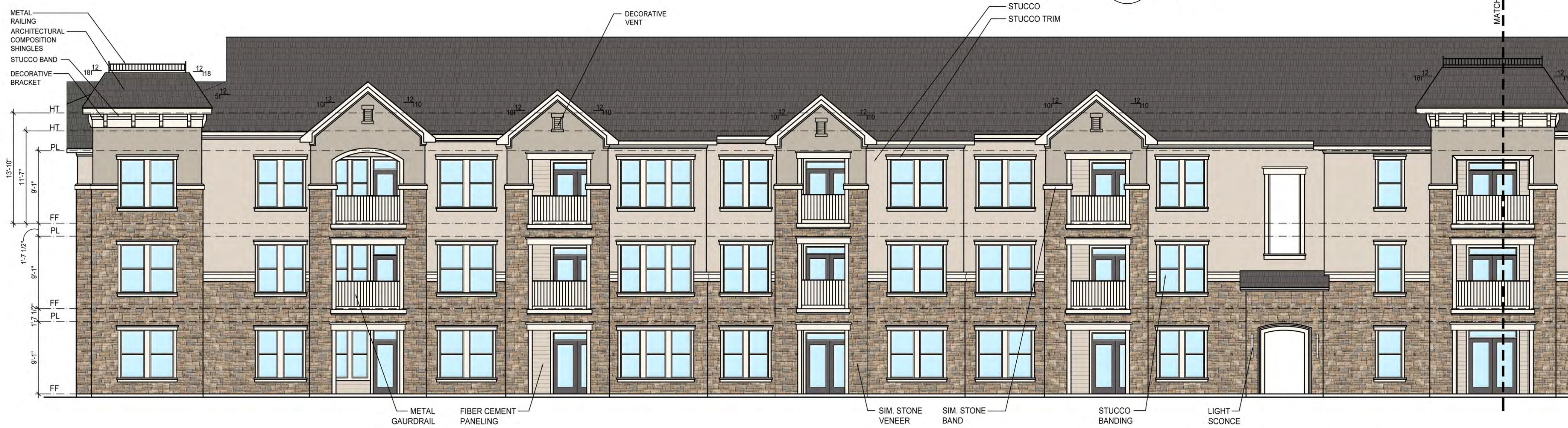
01 BUILDING "G" - REAR ELEVATION 1/8" = 1'-0"
